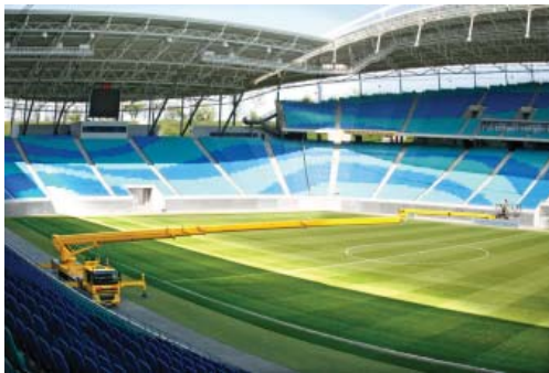
T 580: The most innovative and revolutionary design from Ruthmann, with 58 meters height of stroke and a lateral range of +40 meters.
